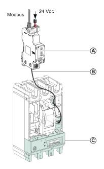
A IFM Modbus SL communication interface for one circuit breaker
