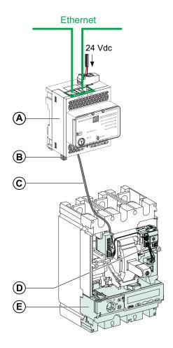
A IFE Ethernet communication interface for one circuit breaker
