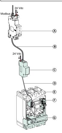
A IFM Modbus SL communication interface for one circuit breaker
