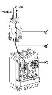
A IFM Modbus SL communication interface for one circuit breaker
