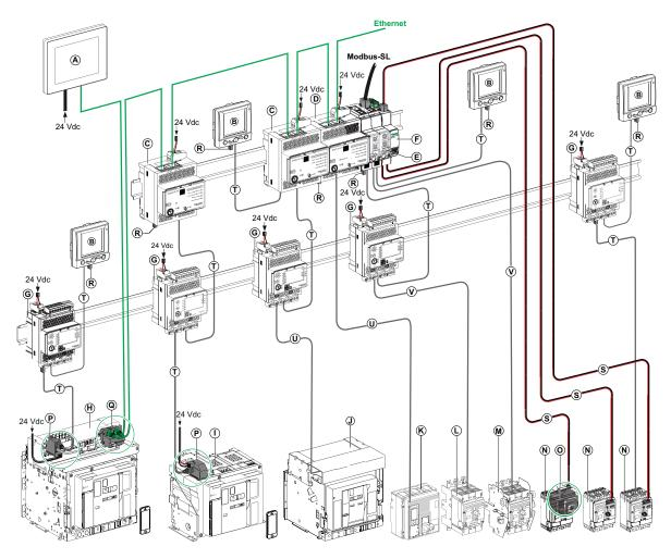
**A** FDM128 Ethernet display for eight devices
