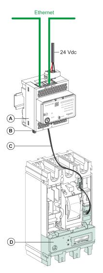
$\ensuremath{\textbf{A}}$  IFE Ethernet communication interface for one circuit breaker
