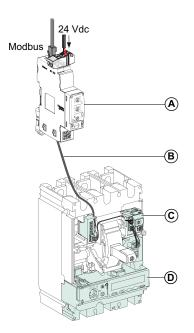
A IFM Modbus SLL communication interface for one circuit breaker
