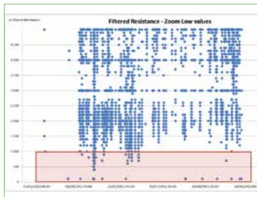
Filtered resistance: There are a few points below 1kOhm that require excellent signal processing and filtering capabilities to avoid undesired tripping.
